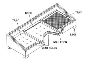
Figure 2: The Brace solar dryer.
