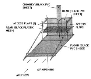
Figure 1: The Exell cabinet solar dryer.
